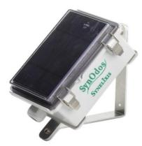
The **SynOdos** is a wireless peripheral monitoring and control device which **connects wirelessly** to a SynField head-node that acts as a gateway. irrigation etc).
