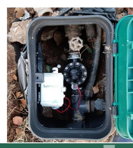
The interconnection between SynField and SynNano device is based on the LoRa wireless technology. The distance between **SynField** head node and **SynNano peripheral** node can reach **up to 3 km**.
